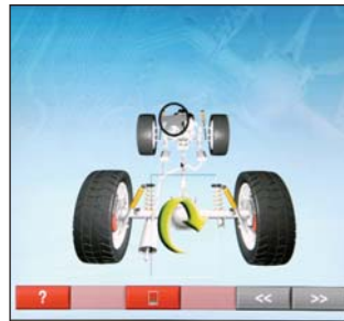
Vehicle run-out on ground or on lift.
