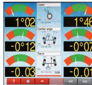
Easy-to-read rear meter provides caster, camber, and toe, all on one screen.
