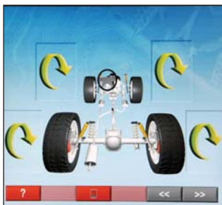
View run-out while vehicle is raised.
